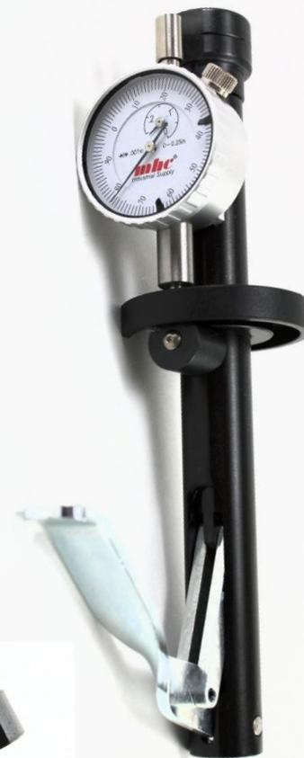
3. Rotate the cam ring back to the home position and release the handle. The dial indicator stem now rests on the primer.
