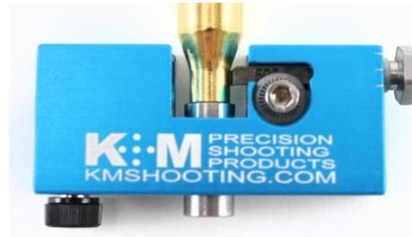
Adjust pilot so cutter tip is close to neck/shoulder junction
