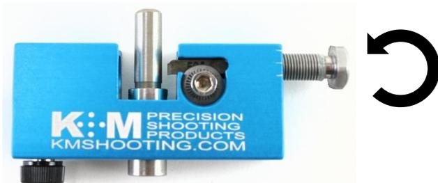
Insert the cutter assembly back into the neck turner body and rotate the adjustment nut COUNTERCLOCKWISE until cutter tip is .025"-.040" from pilot.
